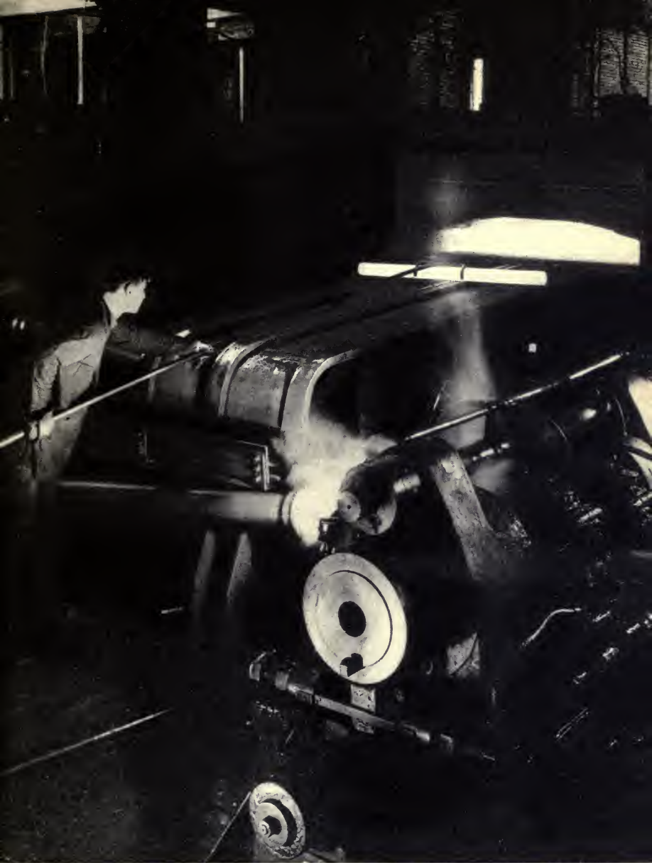
WITHDRAWING A HEATED COPPER BILLET FROM THE FURNACE, AMERICAN BRASS COMPANY, WATERBURY
